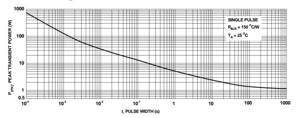
Figure 11. Single Pulse Maximum Power Dissipation
