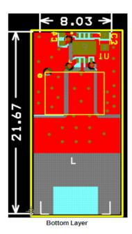
Figure 31. Recommended PCB Layout
