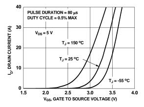
Figure 5. Transfer Characteristics
