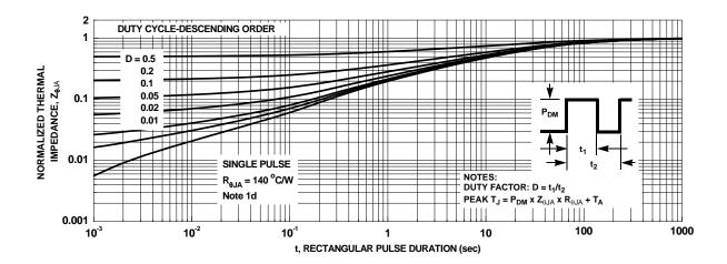
Figure 24. Junction-to-Ambient Transient Thermal Response Curve
