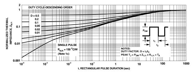
Figure 12. Junction-to-Ambient Transient Thermal Response Curve
