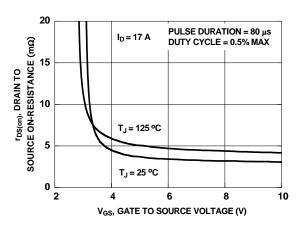
Figure 16. On-Resistance vs Gate to Source Voltage
