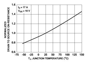
Figure 15. Normalized On-Resistance vs Junction Temperature
