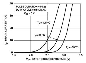
Figure 17. Transfer Characteristics
