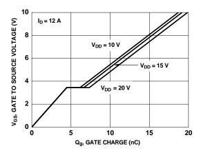
Figure 7. Gate Charge Characteristics
