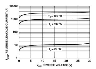
Figure 26. SyncFET<sup>TM</sup> body diode reverse leakage versus drain-source voltage
