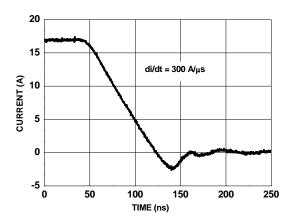
Figure 25. FDML7610S SyncFET<sup>TM</sup> body diode reverse recovery characteristic
