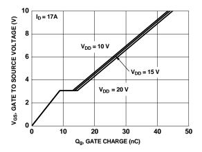
Figure 19. Gate Charge Characteristics
