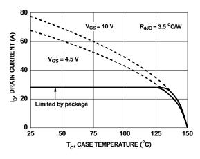
Figure 21. Maximun Continuous Drain Current vs Case Temperature
