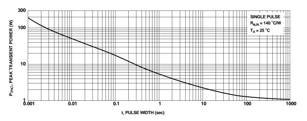
Figure 23. Single Pulse Maximum Power Dissipation
